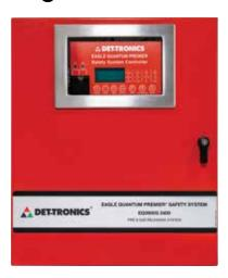
The **Safety System** manages and controls the fire and gas detection/releasing system. It is a listed, configurable, distributed, and intelligent safety system that provides fire and gas detection, alarm signaling, notification, extinguishing agent release, and deluge operation. All system components are integrated together on a fault-tolerant Class X SLC digital communication network. The certified
